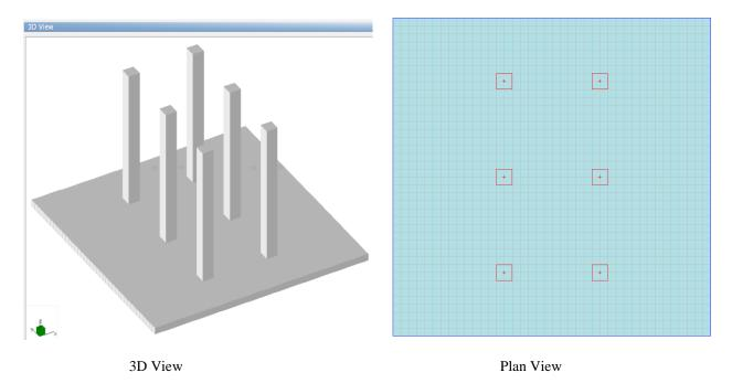
To investigate or design a slab with a single layer or reinforcement, spMats design parameters definition input requires special attention in order to determine the correct area of steel required.
